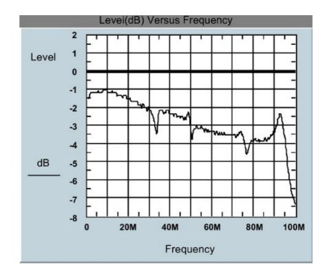
The next coupler used 2 cores wound with 9 turns on each and a wire between output /input forward and reflected. According to the rfcandy chart this should give 18dB coupling with 40dB directivity.
