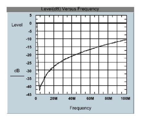
The coupler is barely usable from 5 to 10Mhz. What was the reason for this, too much self capacitance of windings coupling across the core apertures.
