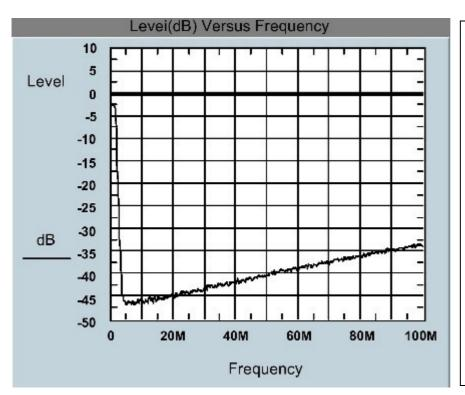
The results for a 2 + 2 turn transformer. This is more like it! The rising characteristic up to 33dB at 100Mhz would probably be due to stray capacitance.
