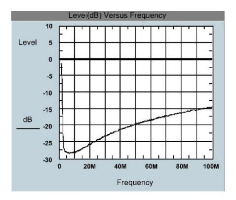
Only 27dB directivity max deteriorating to 15dB at 100Mhz hardly useable. Then a combination of the 2 resistor and coupling transformer design was tried
