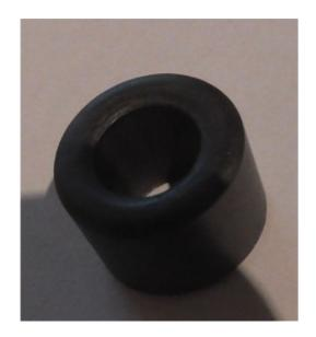
10mm inside diameter 25mm long (a half core is shown here
